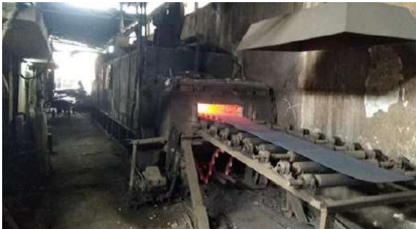
Figure 4.6: Reheating furnace (sheet metal)
