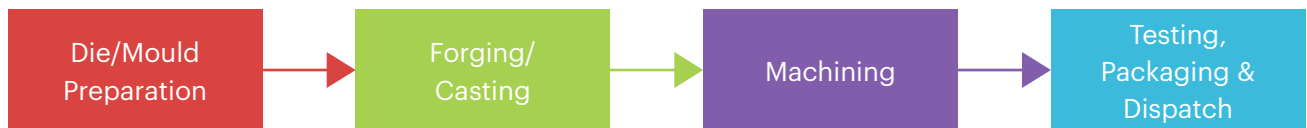
Figure 1.5: Typical production process of engineering equipment
